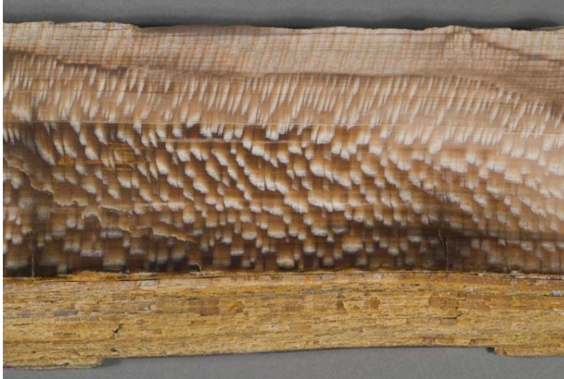
Section of Squaw Creek sycamore cut on radial axis to show the grain pattern
